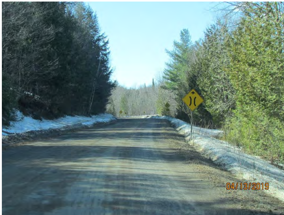
Photo 9 (Looking N): Station 5+400 – On Ferguson Lake Road, approaching the Constant Creek Bridge, insufficient hazard signage and measures to protect traffic convergence at bridge location.
